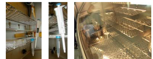
An example of the functionality of the ViVoX TC biosystem. All shelves parts can be autoclaved and replaced. The shelves can also be used for hanging pipettes and test tubes.
